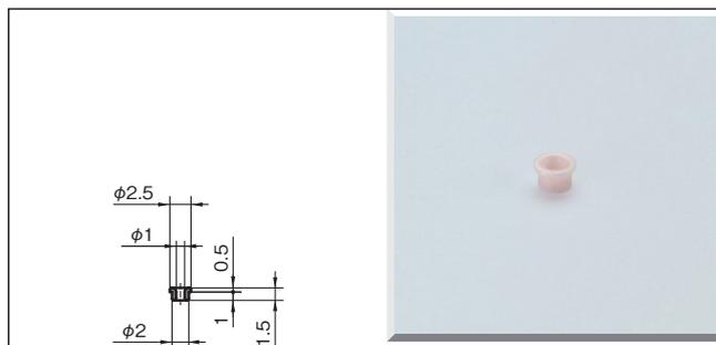
Technical drawing showing dimensions:  $\phi 2.5$ ,  $\phi 1$ ,  $\phi 2$ , 0.5, 1, 1.5.
