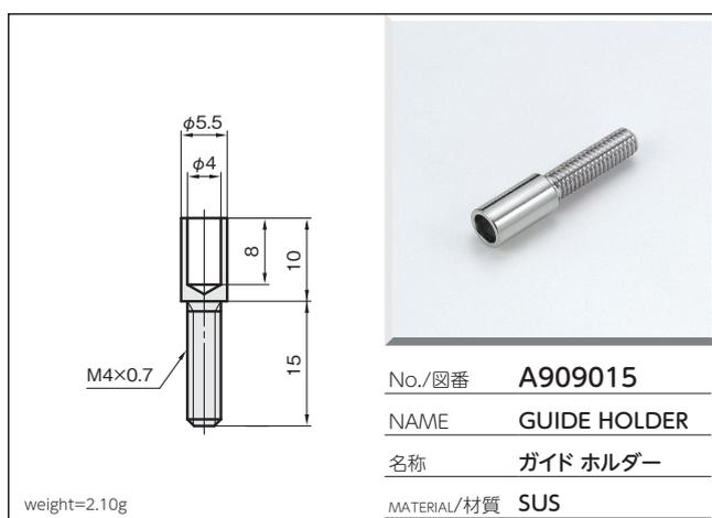
Technical drawing showing dimensions:  $\phi 5.5$ ,  $\phi 4$ , 8, 10, 15, M4x0.7.
