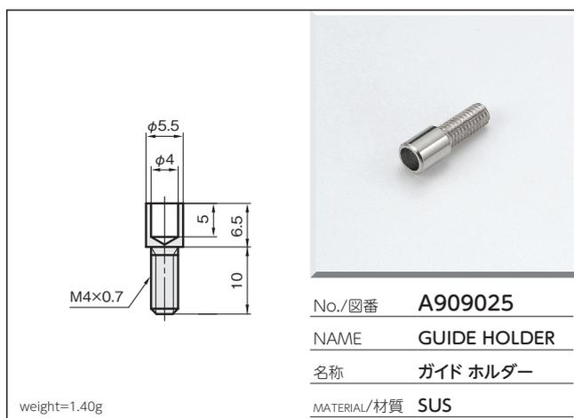
Technical drawing showing dimensions:  $\phi 5.5$ ,  $\phi 4$ , 5, 6.5, 10, M4x0.7.
