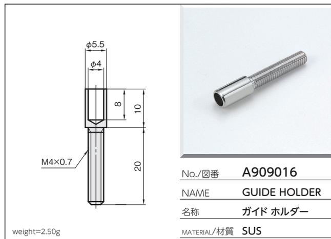
Technical drawing showing dimensions:  $\phi 5.5$ ,  $\phi 4$ , 8, 10, 20, M4x0.7.
