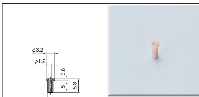
Technical drawing showing dimensions:  $\phi 3.2$ ,  $\phi 1.2$ ,  $\phi 2.2$ , 0.8, 5, 5.8.
