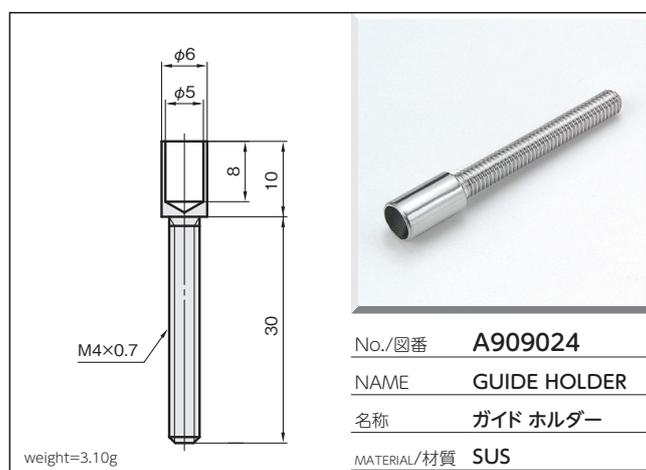
Technical drawing showing dimensions:  $\phi 6$ ,  $\phi 5$ , 8, 10, 30, M4x0.7.
