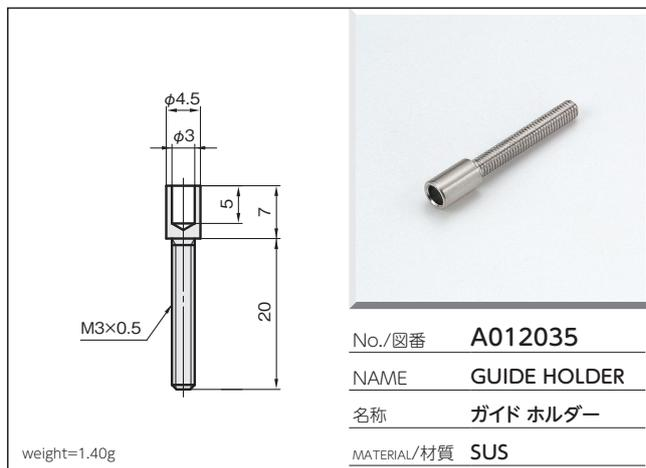
Technical drawing showing dimensions:  $\phi 4.5$ ,  $\phi 3$ , 5, 7, 20, M3x0.5.
