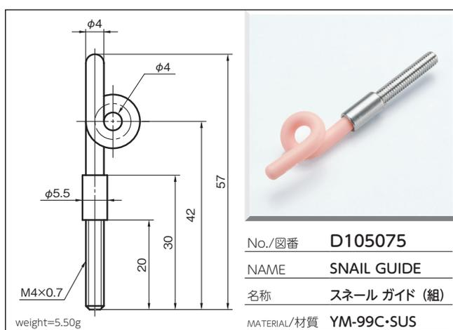
Technical drawing showing dimensions:  $\phi 4$ ,  $\phi 4$ , 57, 42, 30, 20, M4x0.7.
