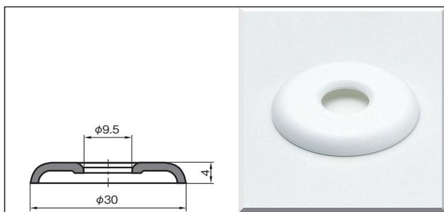
Technical drawing showing dimensions:  $\phi 9.5$  (inner hole),  $\phi 30$  (outer diameter), and 4 (thickness).
