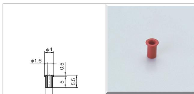
Technical drawing showing dimensions:  $\phi 4$ ,  $\phi 1.6$ ,  $\phi 3$ , 0.5, 5, 5.5.
