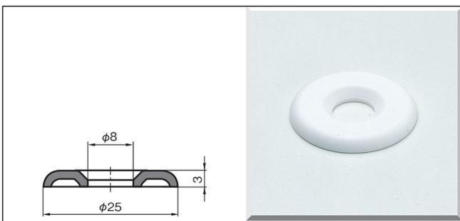
Technical drawing showing dimensions:  $\phi 8$  (inner hole),  $\phi 25$  (outer diameter), and 3 (thickness).
