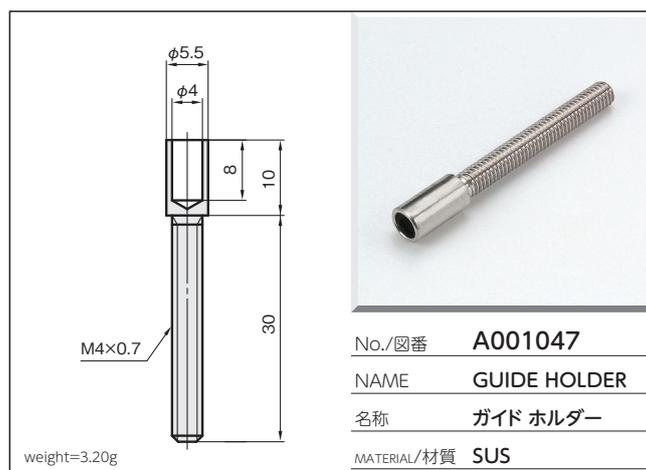
Technical drawing showing dimensions:  $\phi 5.5$ ,  $\phi 4$ , 8, 10, 30, M4x0.7.
