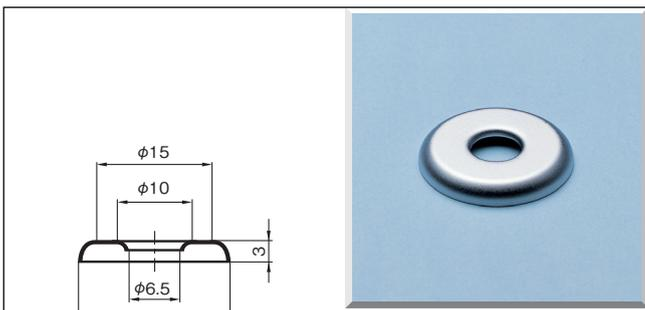
Technical drawing showing dimensions:  $\phi 15$  (outer diameter),  $\phi 10$  (inner hole),  $\phi 6.5$  (inner diameter),  $\phi 20$  (outer diameter), and 3 (thickness).
